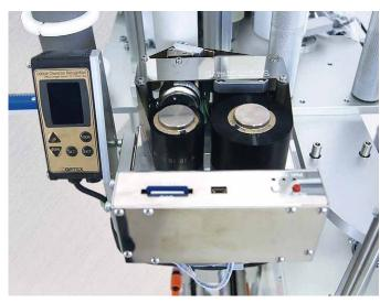
Thermal printer and printing inspection unit can also be installed (Optional).
